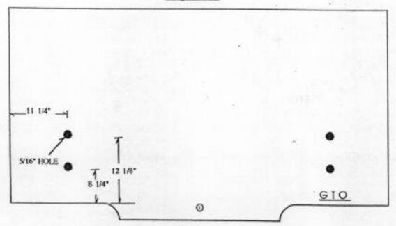
Measurements are taken using the edge of the decklid above the taillights as the starting point. Follow the contour of the decklid with a measuring tape to the correct dimension. Drill a 5/16\* hole for the studs.
